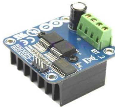
Figura 11 - Driver de Motor BTS7960 (H-Bridge).[17]
