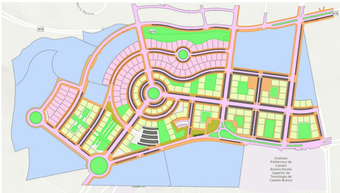
Figure 15: Plots, Buildings, Greenspaces, Public Equipments are shown along with roads, sidewalks and parkings in ArcGIS, represented with color-coded layers as described in the legend below.
