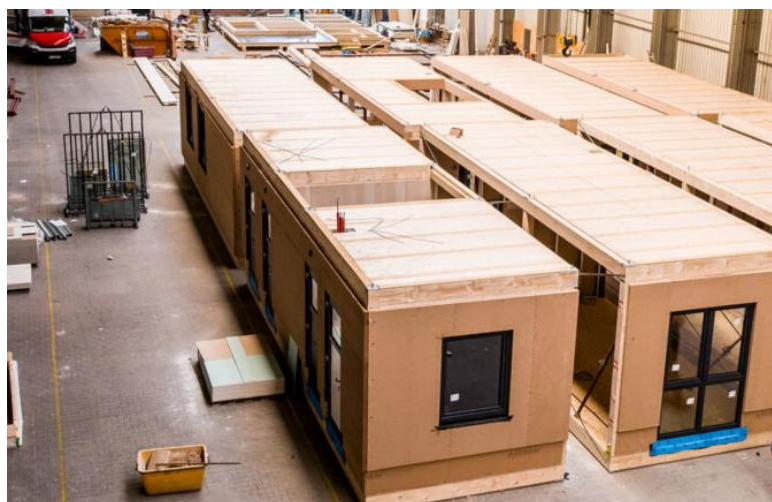
Figure 6.1 — Three-dimensional CLT structure acting as a rigid structural box, illustrating load-bearing walls, floor diaphragms and global structural stability in mid-rise construction.
