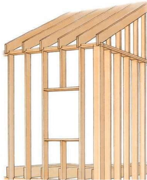
Figure 3.3 — Evolution of timber structural systems: North American balloon frame system, representing the transition towards lightweight, repetitive and industrialised timber construction techniques.
