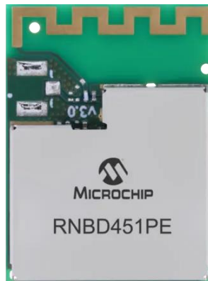
Figura 7- Módulo Bluetooth RNBD451PE, fabricante Microchip Technology [2].
